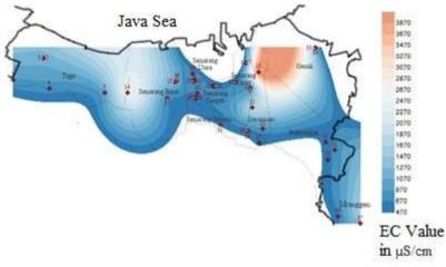
Figure 3. Contours of electrical conductivity (EC) in the research area
