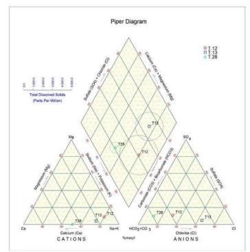
Figure 4. Piper Trillineardiagram resultsplotting groundwater samples shallow wells in the study area
